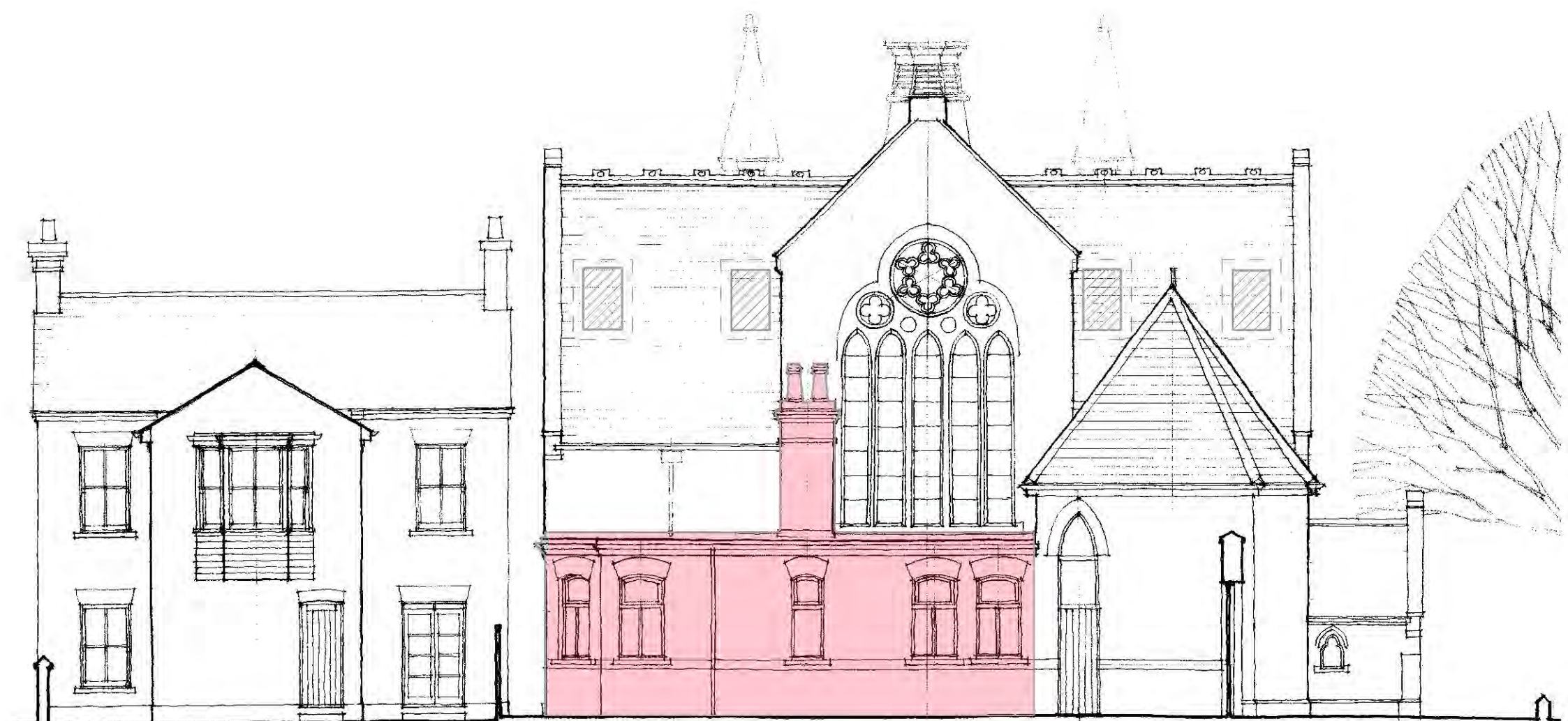
Demolitions West Elevation
